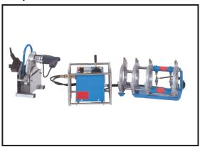
50mm - 160mm (1-1/2" - 6") Size Range Single & Double Wall **Piping** PE, PP, PVDF **Materials** 230 Single **Power**
