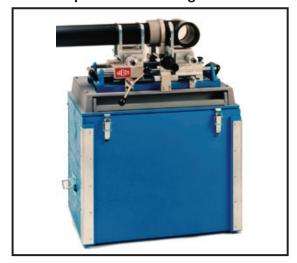
20mm - 110mm (1/2" - 4") Size Range Single Wall **Piping** PE, PP, PVDF **Materials** 110v **Power**
