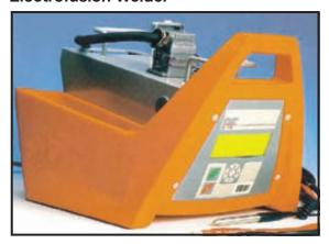
All electrofusion fittings up to 48 volt Size Range Single Wall **Piping** PE, PP **Materials** 110v **Power** 21"x27"x19" **Dimensions**
